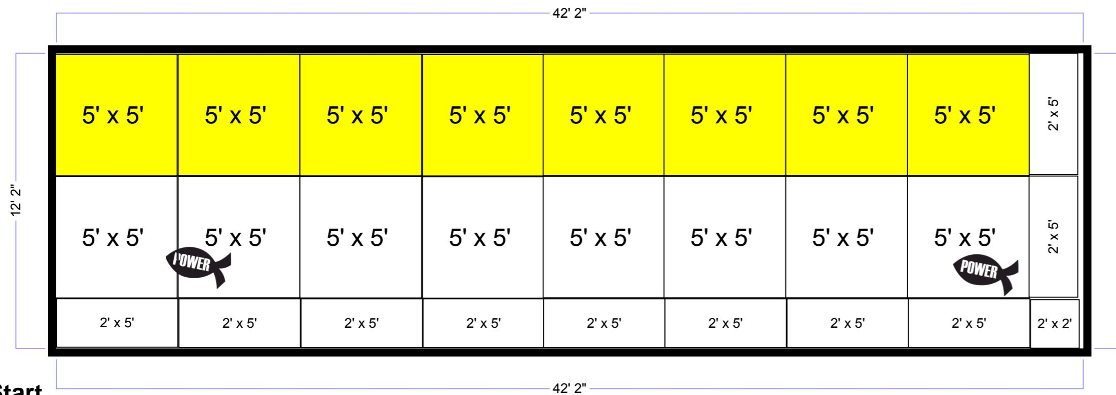
**Instructions:** When laying the top boards start in the corner with the 2'6" x 2'6" and then lay all the highlighted boards.
