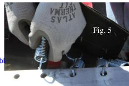
that are sewn along the edges of the bed). Take the first spring in the first D-Ring and attach to the first hole in the rail. You will then take the second spring in the first D-Ring and attach it to the second hole in the rail. (See Fig. 5)
